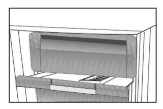
When deep-freezing hot food, the cooling compressor will work until the food is completely frozen. This can temporarily cause excessive cooling of the refrigeration compartment.
